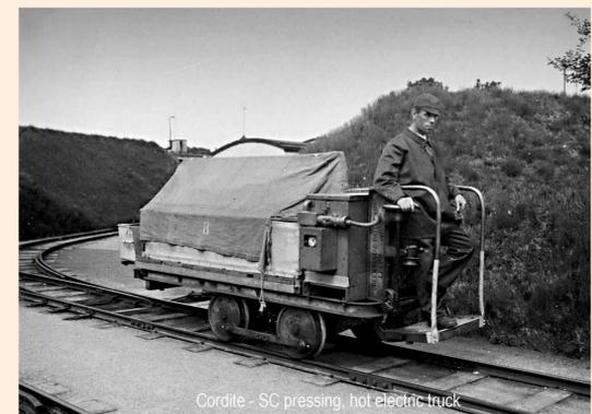
An electric railcar. Steam engines were not used, because sparks could have started fires and explosions. (photo: RNCFA)
